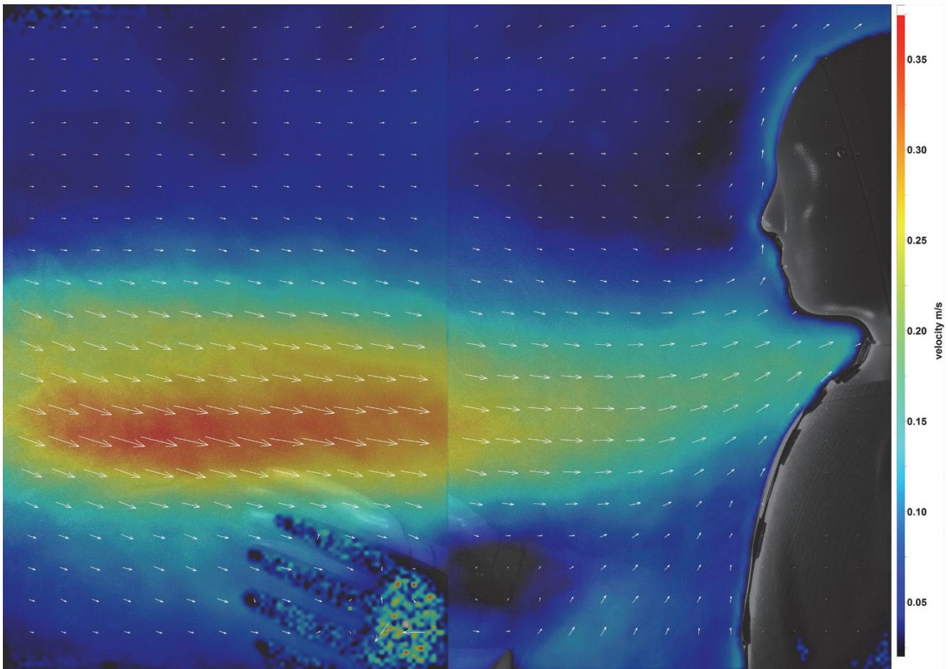
Figure 7 Interaction of the flows with a supply of  $30 \text{ m}^3/\text{h}$
