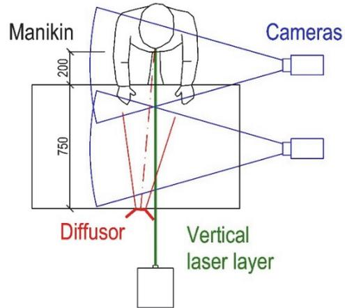
Figure 4 Settings of the flow interaction measurement
