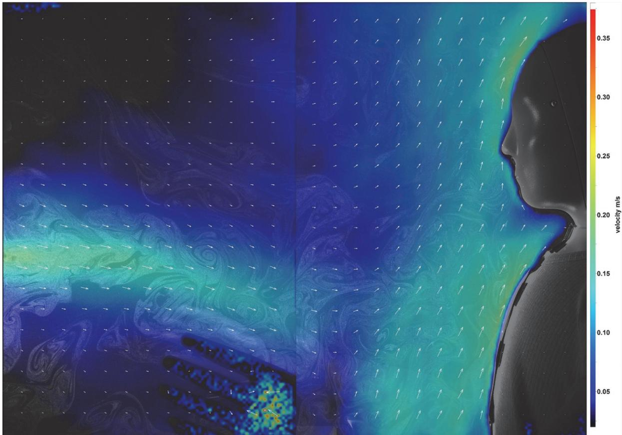
Figure 5 Interaction of the flows with a supply of 15 m<sup>3</sup>/h
