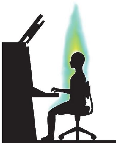
Figure 1 Convective boundary layers around the sitting human body.
