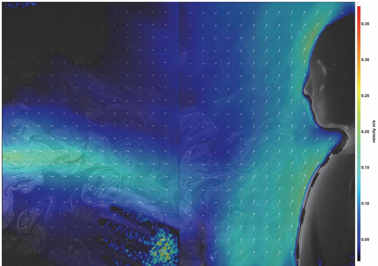
Figure 5 Interaction of the flows with a supply of  $15 \text{ m}^3/\text{h}$
