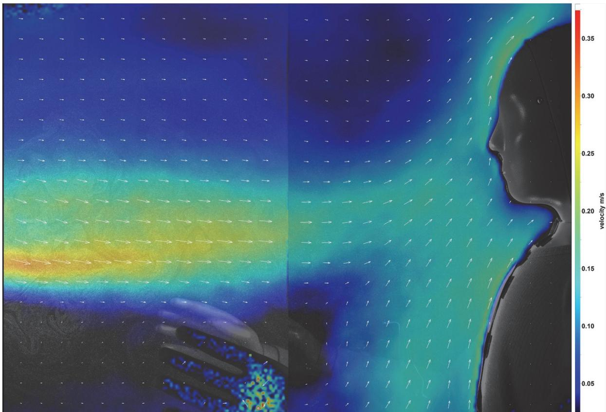
Figure 6 Interaction of the flows with a supply of 25 m<sup>3</sup>/h
