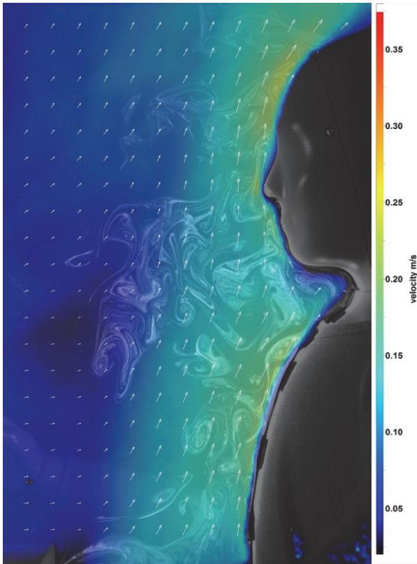
Figure 3 Vector field of the boundary layers
