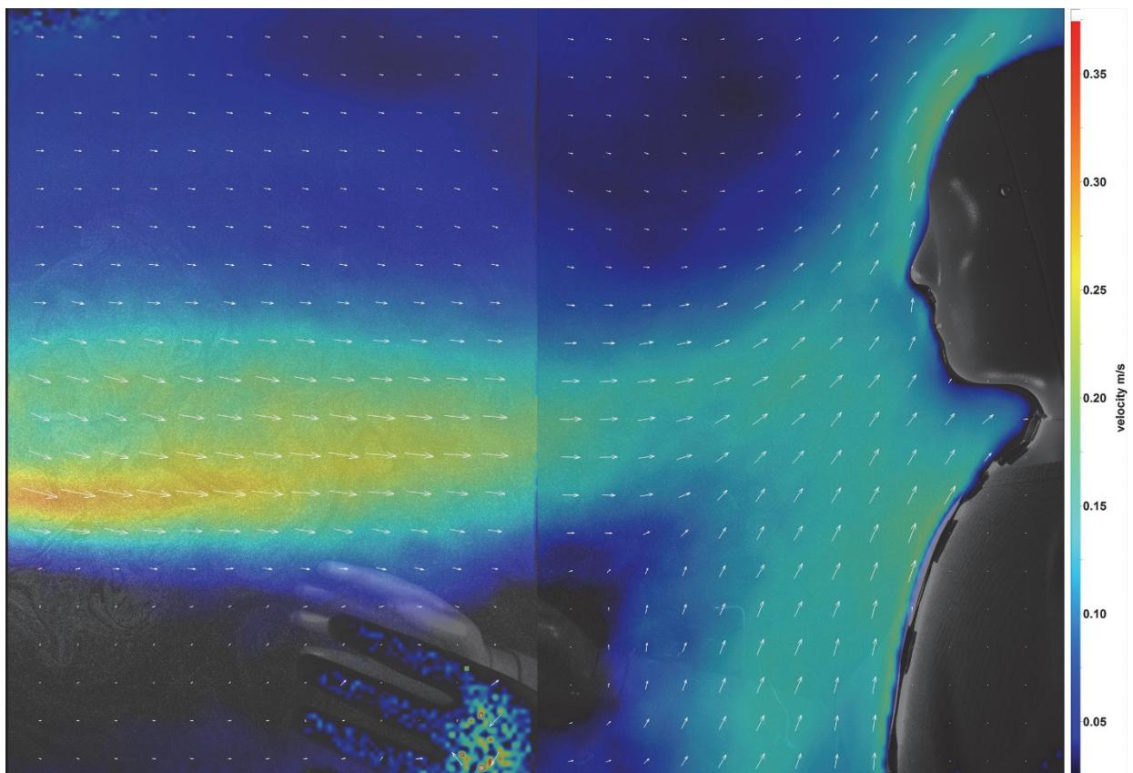
Figure 6 Interaction of the flows with a supply of  $25 \text{ m}^3/\text{h}$
