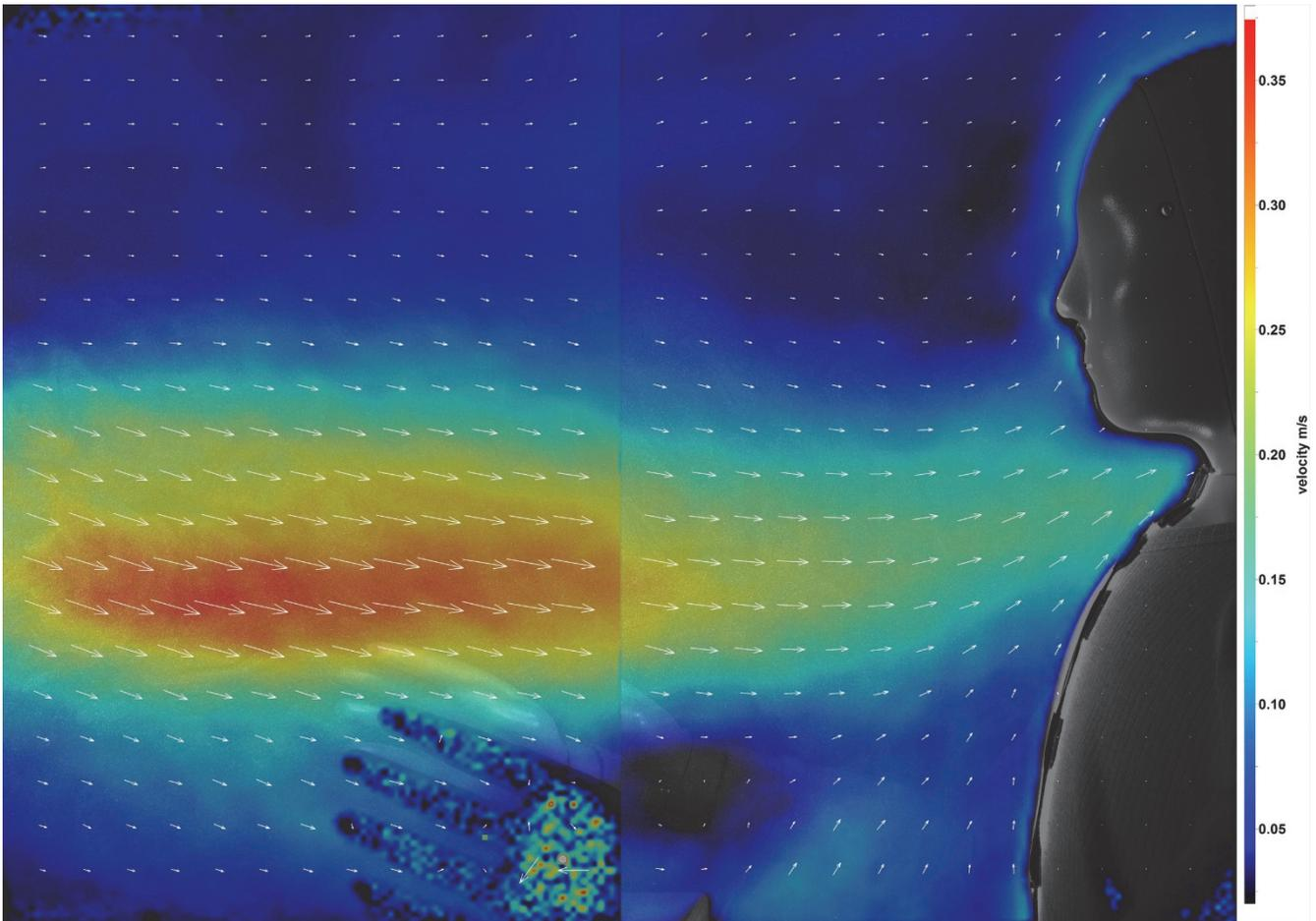
Figure 7 Interaction of the flows with a supply of 30 m<sup>3</sup>/h
