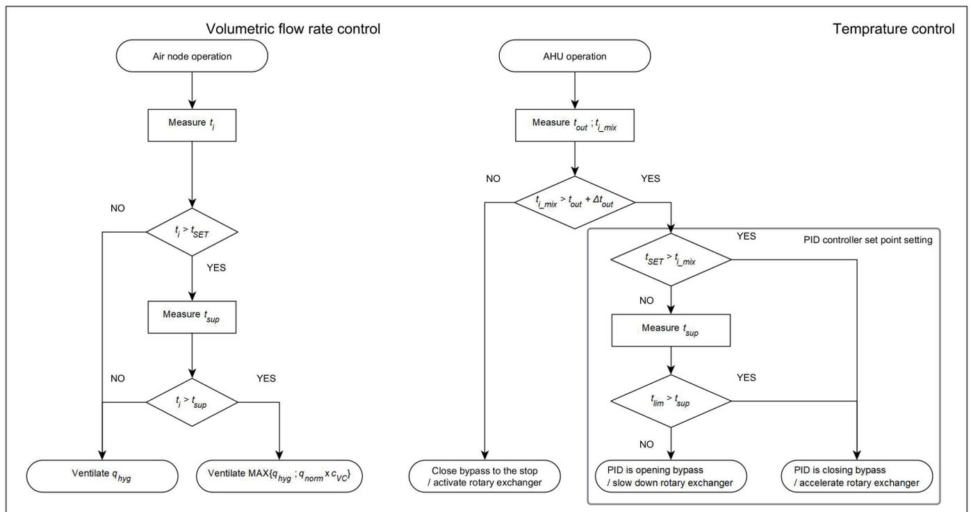
Fig. 1 Ventilative cooling operation flowchart
