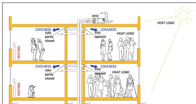
Fig. 2 Cross section of a group of rooms cooled by the ventilation [40].
