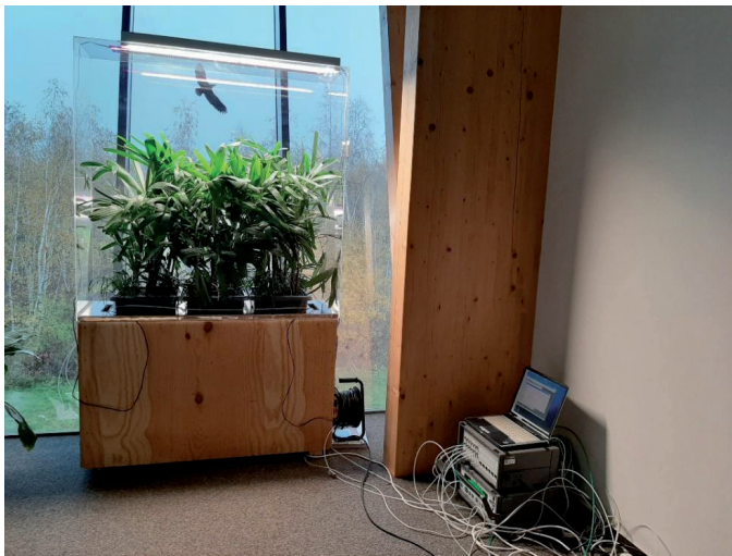
Figure 4 Experimental green partition in a meeting room with an extra Lumasense Innova measuring device for the air analysis
